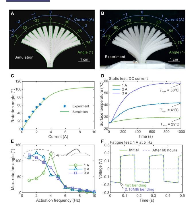
Characterization of a single-coil square SEMA. Rotation angle of the SEMA subjected to a DC current from 1 to 3 A (A) predicted in the simulation and (B) observed experimentally. (C) Rotation angle of the SEMA as a function of the current for experiment and simulation. (D) Temporal change of the surface temperature of the SEMA for three specific values of DC current, 1, 2, and 3 A. (E) Maximum rotation angle of the bending SEMA subjected to square wave
