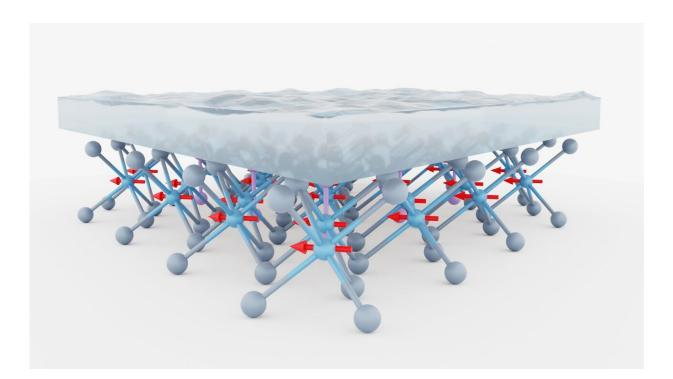
Ball-and-stick model of the crystal structure of Cr2Ge2Te6 covered with the ion gel. The red arrows represent the magnetic moments of Cr atoms. Credit: Verzhbitskiy et al.
