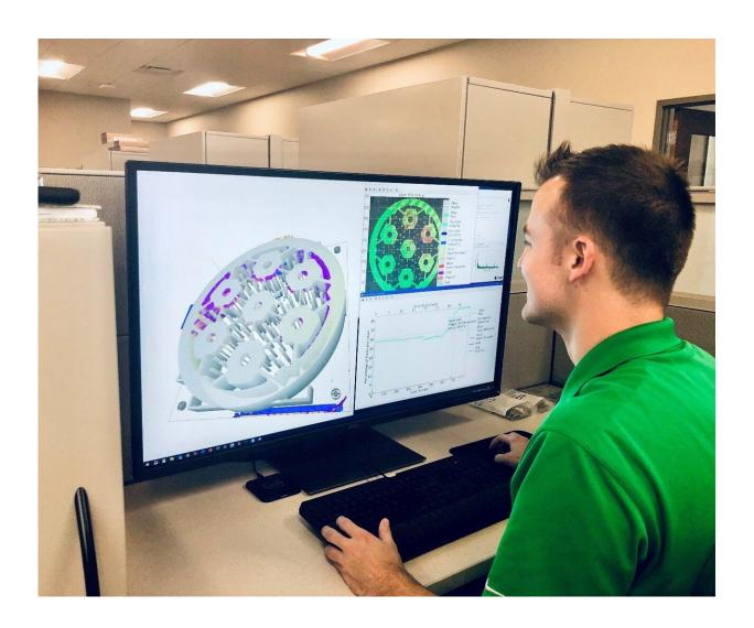
Oak Ridge National Laboratory researcher Chase Joslin uses Peregrine software to monitor and analyze a component being 3D printed at the Manufacturing Demonstration Facility at ORNL. Credit: Luke Scime, ORNL, U.S. Dept of Energy
