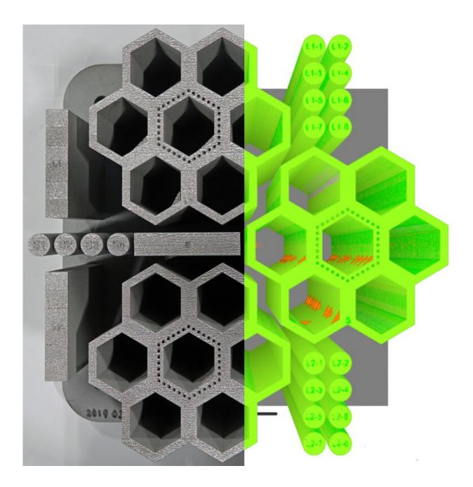
Peregrine detects an anomaly in a component being additively manufactured on a powder bed printer at the Manufacturing Demonstration Facility at ORNL. Credit: Luke Scime, ORNL, U.S. Dept. of Energy
