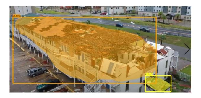
Drone video of damage from Hurricane Laura in Lake Charles, LA, was processed automatically by a Carnegie Mellon University system. Areas bounded in orange are considered severely damaged, while those in yellow are slightly damaged. Credit: Carnegie Mellon University
