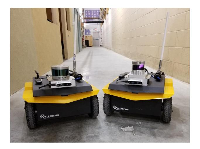
The two robots used in the experiments are identically equipped, with the exception of Velodyne VLP-16 LiDAR (left) and Ouster OS1 LiDAR (right). Credit: U.S. Army photo
