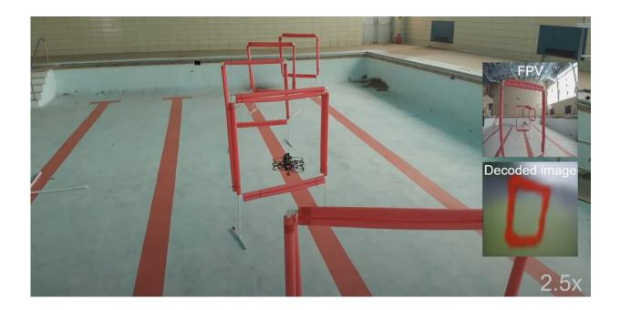
To fly autonomously, drones need to understand what they perceive in the environment and make decisions based on that information. A novel method developed by Carnegie Mellon University researchers allows drones to learn perception and action separately. The two-stage approach overcomes the "simulation-to-reality gap," and creates a way to safely deploy drones trained entirely on simulated data into real-world course navigation.
