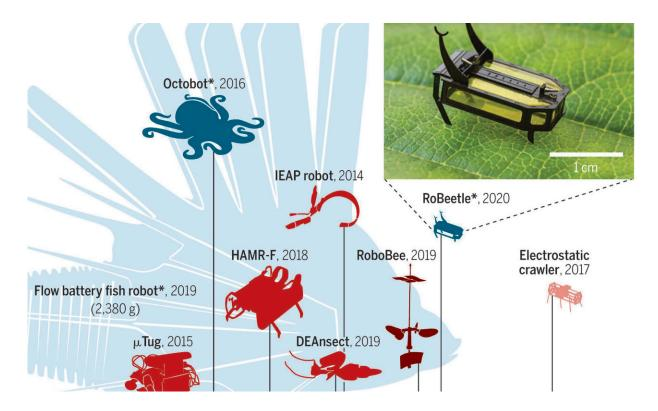
Comparison of various untethered microrobots and bioinspired soft robots that use different power and actuation strategies. Credit: A. Kitterman/Science Robotics from R.L.T./MIT
