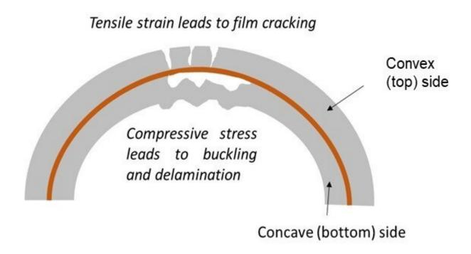
A diagram of how tensile strain leads to the film cracking. Credit: University of Warwick
