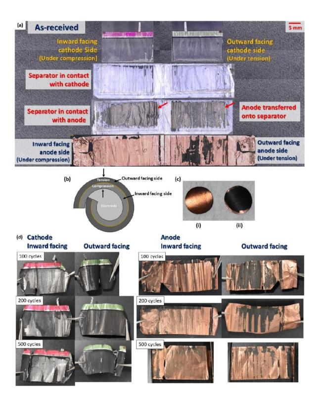
An image demonstrating the stresses to anodes and cathodes after cycles. Credit: University of Warwick
