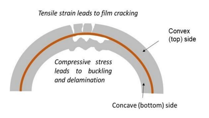
A diagram of how tensile strain leads to the film cracking. Credit: University of Warwick
