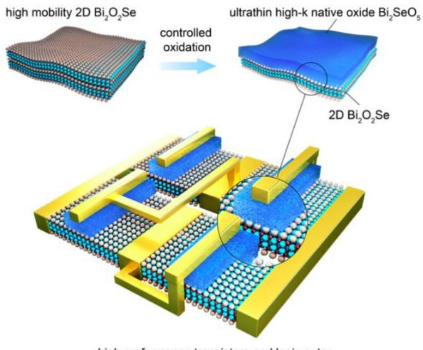
high performance transistors and logic gates
