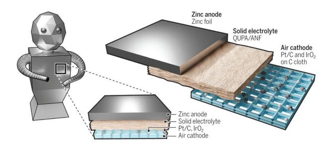
Schematic of a structural Zn-air battery and an example of how it could be used to provide structure to a robot. Credit: Alice Kitterman / Science Robotics
