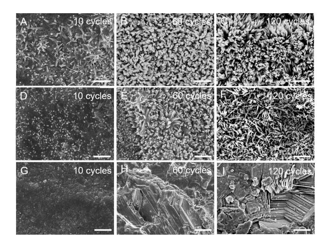
Scanning electron microscopy images of the surface of zinc electrode after going through a certain number of cycles. Credit: Wang et al., Sci. Robot. 5, eaba1912 (2020)
