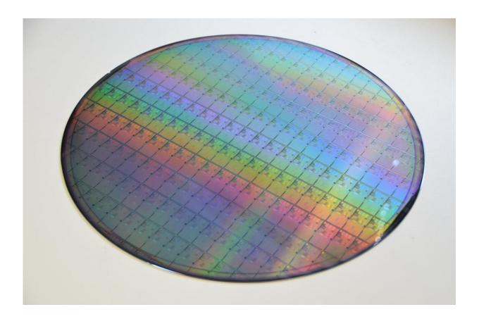
A wafer filled with memristors. Credit: UCL
