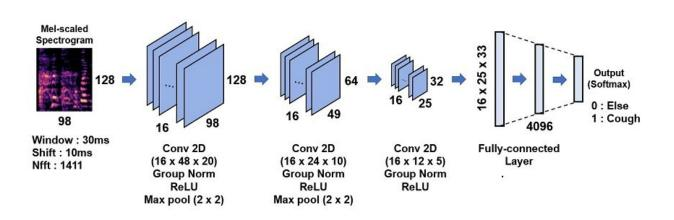
Figure 1. Architecture of the cough recognition model based on CNN. Credit: The Korea Advanced Institute of Science and Technology (KAIST)
