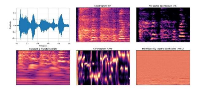
Figure 2. Examples of sound features used to train the cough recognition model. Credit: The Korea Advanced Institute of Science and Technology (KAIST)
