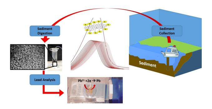
Sediments collected by a ship can be rapidly tested for toxic lead with a new portable lab-on-a-chip device. The miniature device extracts lead from a sample and purifies it, using graphene oxide as a lead detector. Credit: Azam Gholizadeh
