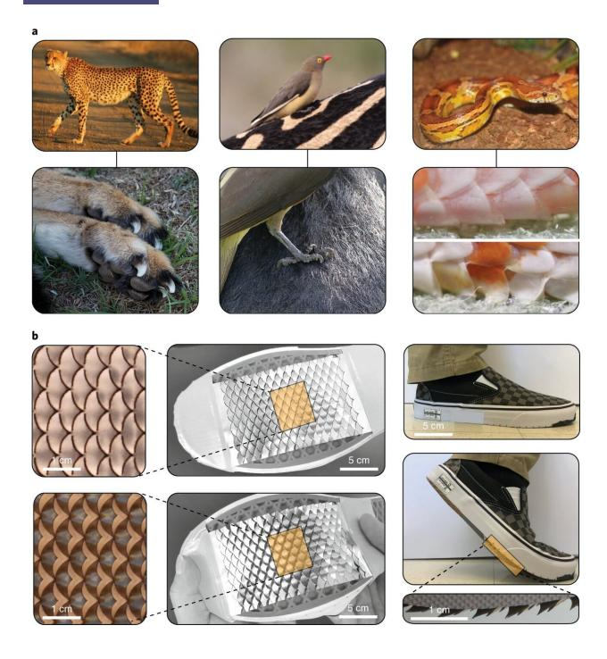
a, Inspiration from friction-enhancing strategies in animals: cheetah with semiretractable claws (left), oxpecker with sharp claws in opposing directions (middle) and snake with scales that are oriented to increase friction (right). b, Kirigami for friction modulation in footwear. Steel kirigami surfaces were attached to the shoe soles (middle). The undeformed (top) and deformed (bottom) configurations of the kirigami shoe grip are illustrated. The spikes are
