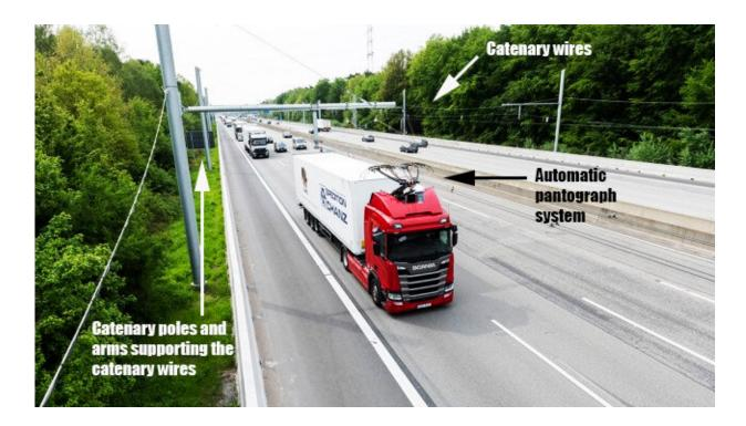
A Scania HGV operating on a catenary lorry 'eHighway' demonstrator in Germany. Credit: Siemens
