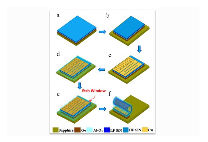
The device-fabrication process includes the deposition of metals by electronbeam evaporation and lithography to define the metal pattern and etching process. The final etching step then triggers the self-rolling process of the stacked membrane. Credit: Xiuling Li.
