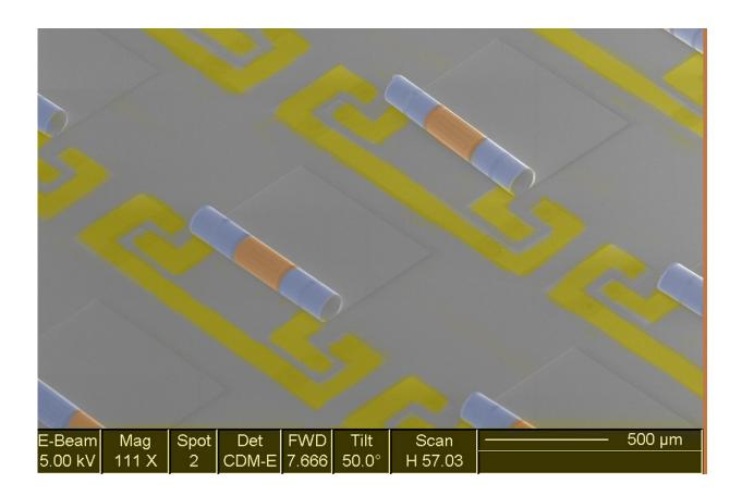
Electron microscope image of an array of new chip components that integrate the inductors, blue, and capacitors, yellow, needed to make the electronic signal filters in phones and other wireless devices. Credit: Xiuling Li
