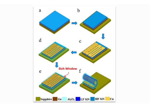
The device-fabrication process includes the deposition of metals by electronbeam evaporation and lithography to define the metal pattern and etching process. The final etching step then triggers the self-rolling process of the stacked membrane. Credit: Xiuling Li.
