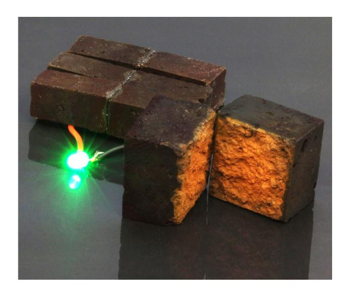
Red brick device developed by chemists at Washington University in St. Louis lights up a green light-emitting diode. The photo shows the core-shell architecture of a nanofibrillar PEDOT-coated brick electrode. Credit: D'Arcy laboratory, Department of Chemistry, Washington University in St. Louis
