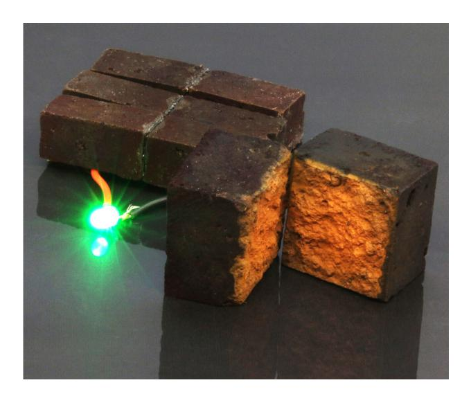
Red brick device developed by chemists at Washington University in St. Louis lights up a green light-emitting diode. The photo shows the core-shell architecture of a nanofibrillar PEDOT-coated brick electrode. Credit: D'Arcy laboratory, Department of Chemistry, Washington University in St. Louis
