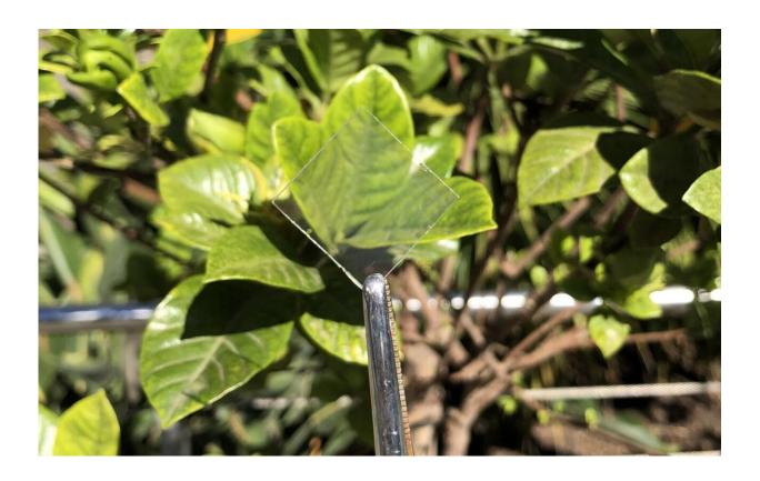
The ultra-thin clear coatings are made with a new spray-on method that is fast, cost-effective and scalable. Credit: RMIT University
