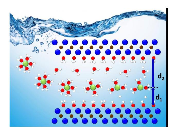
Charged ions, shown in green, move into ultra-thin layers of energy storage materials, shown as blue and brown dots, but are difficult to locate. A holistic approach to track the ions yielded knowledge useful toward improved energy storage devices. Credit: Nina Balke/ORNL, U.S. Dept. of Energy
