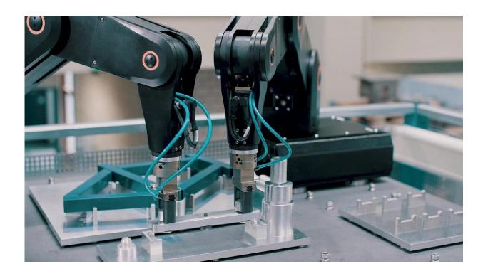
Flexible production system: Higher force and precision, for example when assembling a bicycle frame. Credit: wbk, KIT
