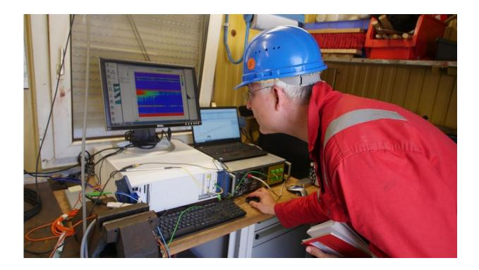
Real-time monitoring during drilling with fiber optic temperature measuring. Credit: CCBY-SA 4.0 Daniel Acksel, GFZ
