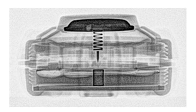
X-ray imaging of the VS-50 antipersonnel landmine shows the unique metal features inside Vibration-ENhanced Underground Sensing system, VENUS, that discriminates between explosives and clutter. Credit: US Army
