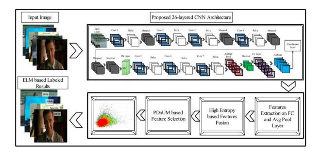
The architecture for human action recognition based on a 26-layer CNN and PDaUM approach proposed by the researchers. Credit: Khan et al.
