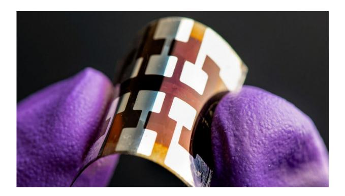
A solar cell made with perovskite, shown here, show promise as an energyefficient, scalable and longer-lasting way to create solar panels. Credit: Dennis Schroeder/National Renewable Energy Laboratory
