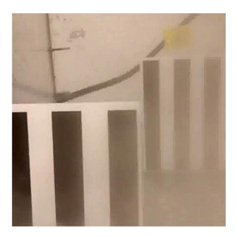
Researchers at Purdue University have developed an image- and video-based application using OpenCV algorithms that detect explosible suspended dust concentration. The app uses a camera or a video recording device to image and determine suspended dust, as well as accurately distinguish it from normal background noise. Credit: Kingsly Ambrose/Purdue University
