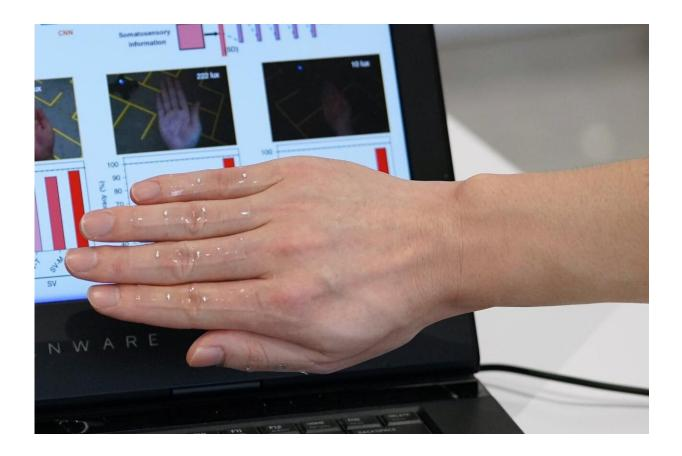
The team fabricated a transparent, stretchable strain sensor that adheres to the skin but cannot be seen in camera images. Credit: NTU Singapore
