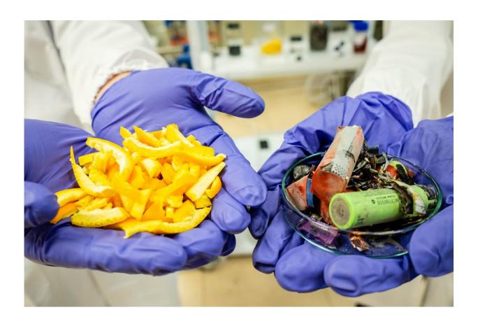
The team demonstrated their concept using orange peel, which recovered precious metals from battery waste efficiently. They then made functional batteries from these recovered metals, creating minimal non-toxic waste in the process. Credit: NTU Singapore
