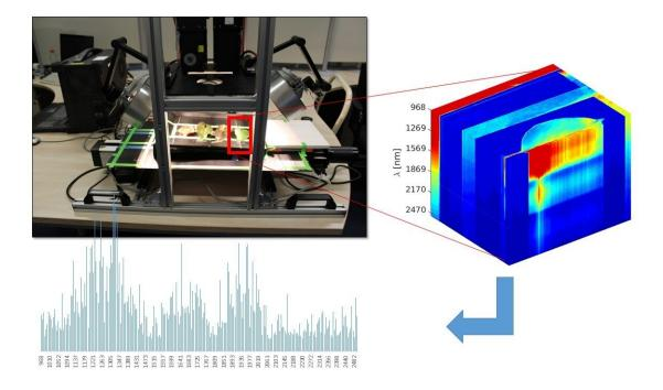
Leaf samples being scanned by hyperspectral cameras in a laboratory. The analysis of image data by machine learning allows conclusions about wavelengths essential to symptom detection, thus enabling the development of optical analysis methods adapted for use in the field. Credit: Uwe Knauer/Fraunhofer IFF
