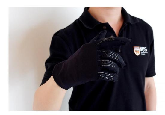
The glove is embedded with thread-line microsensors to produce accurate threedimensional positions of a moving hand, allowing users to mimic a variety of ingame controls using simple gestures. Credit: National University of Singapore
