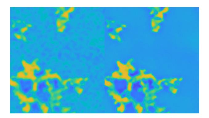
Left and right show false-colored electron microscopic images of the same region on the specimen. But the image on the right has been super resolved using Dr. Yu Ding's new image processing method. Credit: Texas A&M University College of Engineering
