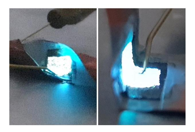
The flexible micro LEDs can be twisted (on left) or folded (on the right). The LEDs, which can be peeled off and stuck to almost any surface, could help pave the way for the next generation of wearable technology. Credit: University of Texas at Dallas
