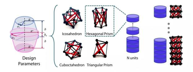
The types of units and how these unit tensegrities are assembled decide the structure-level mechanics of the resulting tensegrity.
