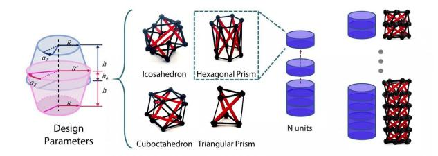
The types of units and how these unit tensegrities are assembled decide the structure-level mechanics of the resulting tensegrity.
