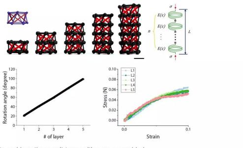
The types of units and how these unit tensegrities are assembled decide the structure-level mechanics of the resulting tensegrity.
