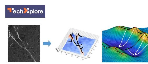
How the "virtual neuroanatomist" traces axonal connections. Though the human eye is good at filling in small gaps in lines to trace axons, computers have trouble with the task. Topological methods help the computer fill in gaps by turning what it sees into a 3D map filled with mountains and valleys. The computer then calculates likely paths from mountaintop to mountaintop. Credit: Mitra lab/CSHL, 2020
