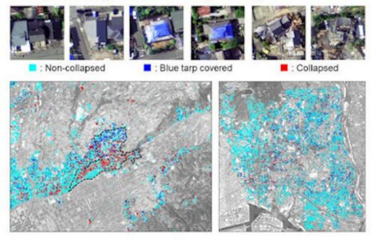
The distribution of damage estimated by the convolutional neural network model for Mashiki town in the 2016 Kumamoto earthquake (L) and Nishinomiya City in the 1995 Kobe earthquake (R). Hiroshima University researchers created a post-disaster damage assessment CNN model that does not need pre-disaster images to make an evaluation. Credit: Hiroyuki Miura
