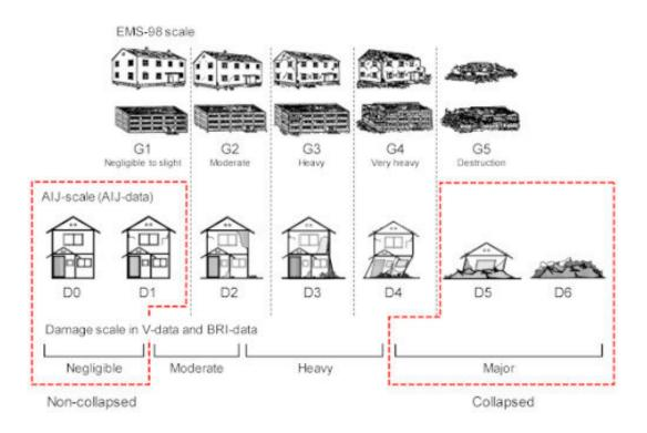
A comparison of the damage scales used by the Architectural Institute of Japan or AIJ scale and the European Macroseismic Scale or EMS-98. Hiroshima University researchers trained the AI to classify D0-D1 damage as non-collapse while D5-D6 is interpreted as collapsed. Credit: Hiroyuki Miura
