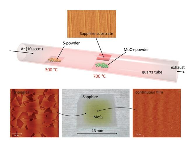
Schematic of the furnace setup used for the CVD growth of our MoS2 films. The process results in almost 1 cm2 film of MoS2 on the sapphire substrate. The isolated monolayer single crystal triangular grains of MoS2 formed on the outer edges of the growth substrate quickly get denser and coalesce into a continuous film of monolayer MoS2 towards the inner part of the sample. Credit: Polyushkin et al.
