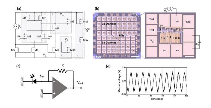
a) Opamp circuit; b) Optical micrograph of the chip, consisting of 64 opamps and test transistors; c) Sketch of the photodetection circuit; d) Output voltage signal from the detection circuit with illumination by incandescent lamp. Credit: Polyushkin et al.
