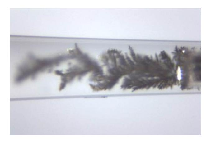
Research from the lab of Peng Bai found that by expanding channels, you can delay and even avoid the formation of dendrites, which can lead to a battery shorting out. The precise relationship can be expressed in terms of a single number, which indicates whether a battery is in danger of shorting, and if so, when. This image is of an expanding channel, which results in a safer battery. The channel widens from about 90  $\mu$ m to about 180  $\mu$ m. Credit: Bai lab
