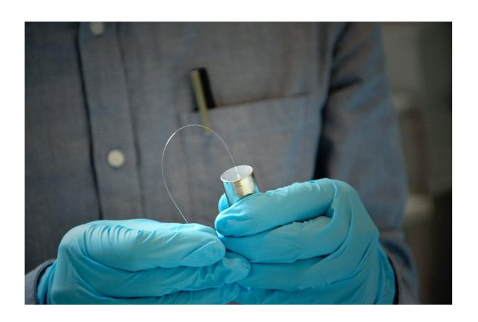
An optical fibre sensor (about 150 microns in diameter) is inserted into a cylindrical cell (18650 format). By placing the optical fibre directly into the center of the cell, the sensor can monitor internal temperature and pressure with unprecedented accuracy. Credit: Collège de France - Benjamin Campech, RS2E.
