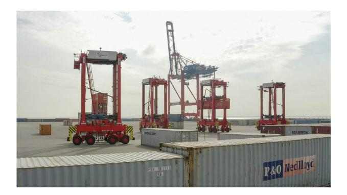
Automated straddle carriers at the container terminal in Wilhelmshaven – efficient and secure. Credit: EUROGATE
