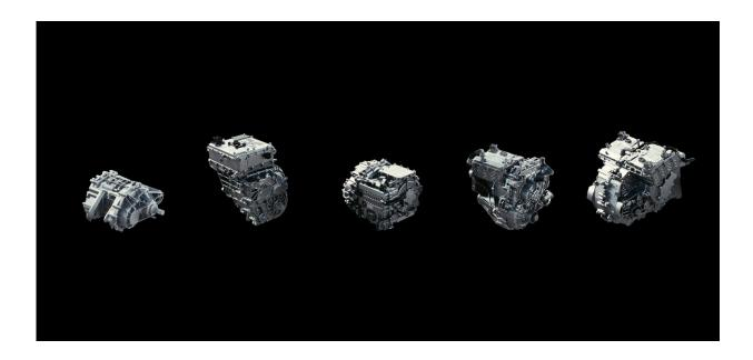
General Motors' next-generation EVs are expected to be powered by a family of five interchangeable drive units and three motors, known collectively as "Ultium Drive.". Credit: GM
