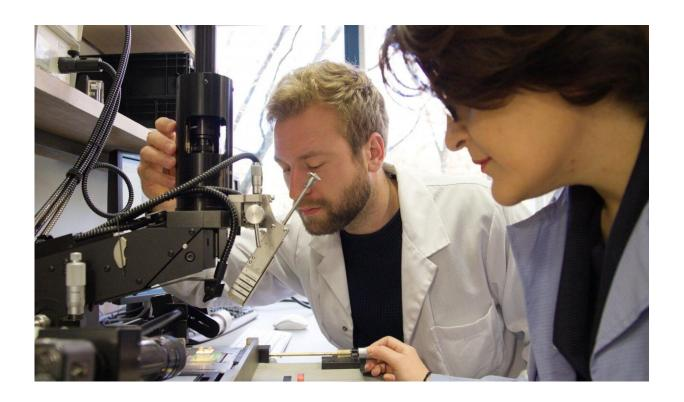
Sevda Abadpour and Axel Diewald from KIT's Institute of Radio Frequency Engineering and Electronics (IHE) place a chip onto a board. Components in the micrometer range have to be aligned perfectly. (Photo: Joachim Hebeler, KIT) Credit: Joachim Hebeler, KIT
