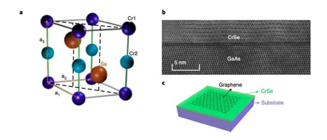
Characterization of the AFM and graphene/AFM heterostructure. A) Crystal structure of the NiAs-phase CrSe. The three lattice vectors are denoted by a1, a2 and a3. The two sublattices of Cr atoms are denoted by Cr1 and Cr2, respectively. B) Transmission electron microscopy side view of the AFM/GaAs, showing the good quality of the AFM. C) A figure showing a graphene/AFM heterostructure. Credit: Wu et al.
