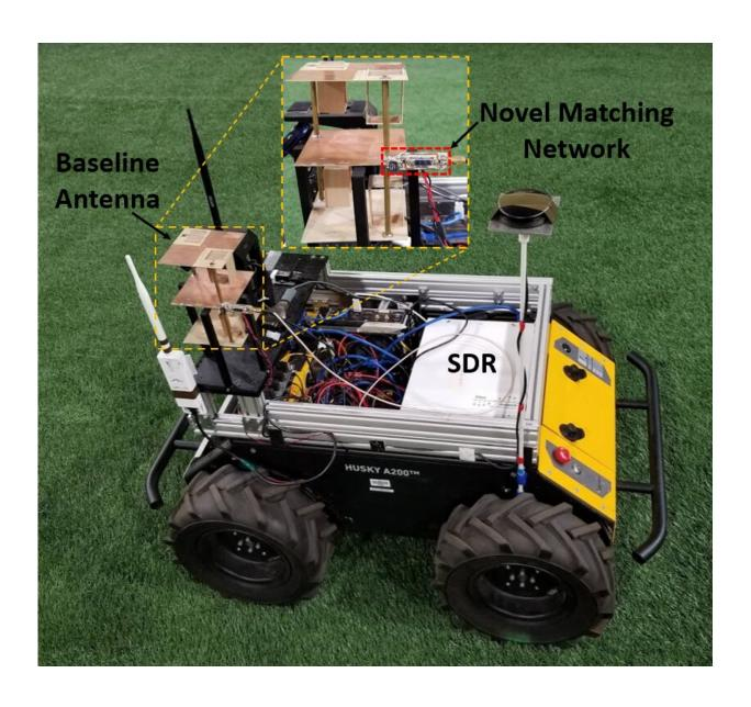
The prototype miniature antenna is integrated on an unmanned ground vehicle
