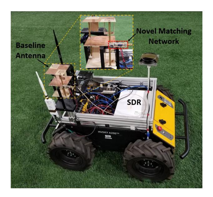
The prototype miniature antenna is integrated on an unmanned ground vehicle
