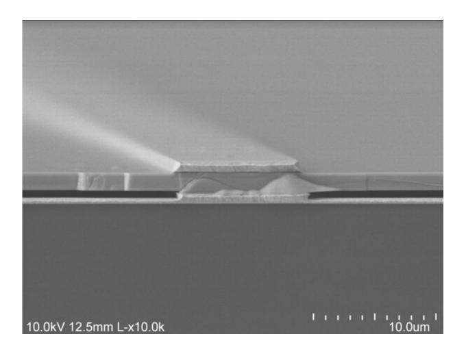
The electron microscope image shows the air (darkest gray) sandwiched between the gold backing at the bottom and the semiconductor at the top, supported on gold beams. Credit: Dejiu Fan, Optoelectronic Components and Materials Group, University of Michigan
