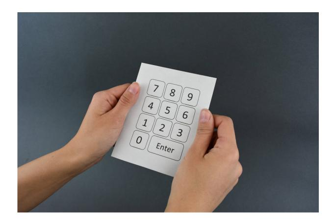
Purdue engineers developed a simple printing process that renders any paper or cardboard packaging into a keyboard, keypad or other easy-to-use humanmachine interfaces. Credit: Purdue University/Ramses Martinez
