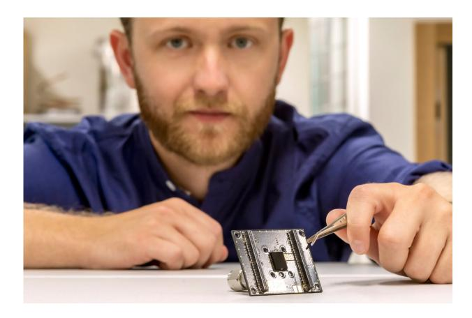
Paul Maierhofer with the result of his dissertation at the Institute for Electrical Measurement and Sensor Technology at Graz University of Technology: the 12 x 9 x 3 millimetre small particle sensor. Credit: Lunghammer - TU Graz
