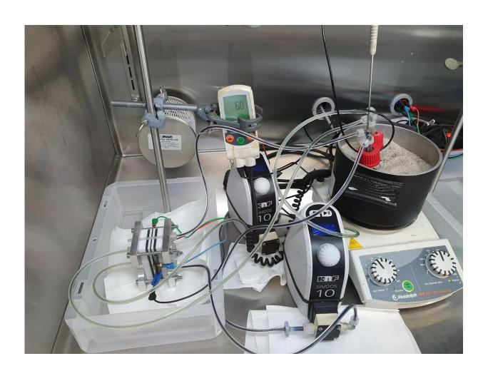
Test setup at CEEC Jena to develop novel active materials for redox flow batteries. Credit: Philipp Borchers/University of Jena
