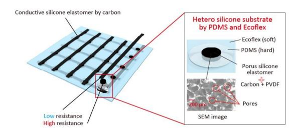
Schematic of the array. This silicone substrate is made of two different silicone types with different hardness values. Harder silicone, PDMS, in the pressure part can suppress the deformation of the pressure sensing elements during tension. Credit: Hiroki Ota, Yokohama National University
