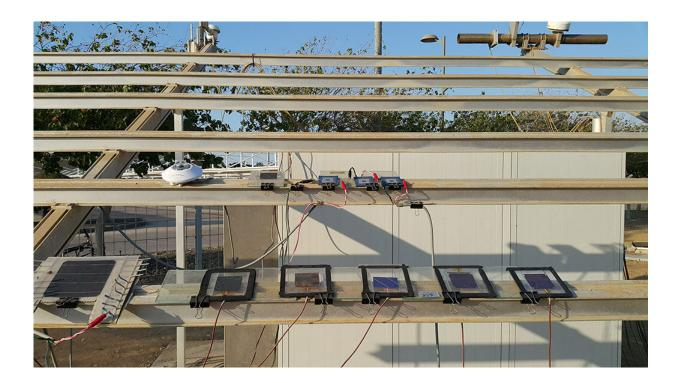
Encapsulated perovskite/silicon tandem solar cells under testing at a KAUST
