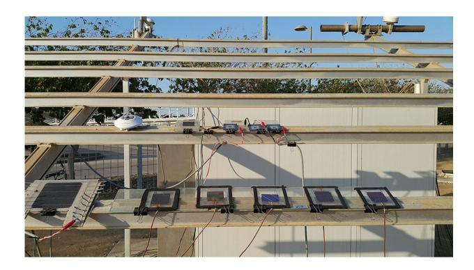
Encapsulated perovskite/silicon tandem solar cells under testing at a KAUST
