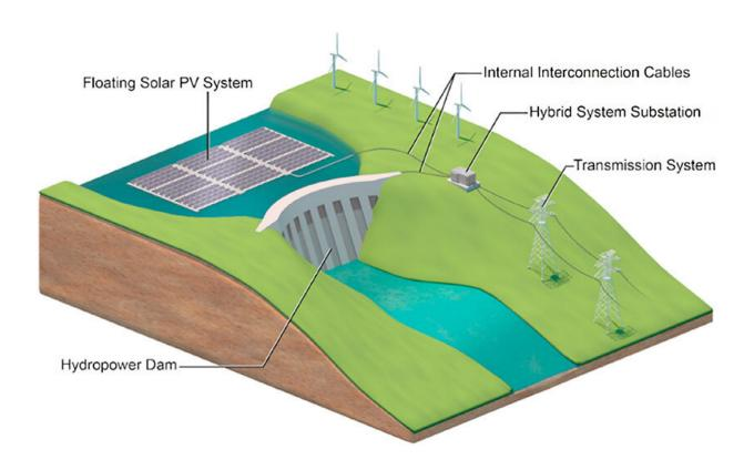
Rendering shows a schematic of a hybrid floating PV-hydropower system. Credit: National Renewable Energy Laboratory
