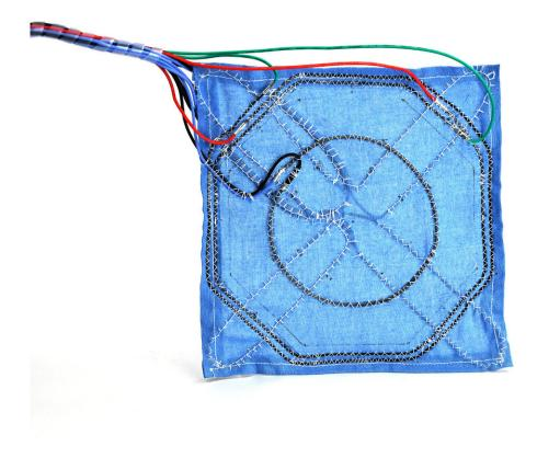
Top-down image of a robotic fabric with integrated actuation, variable stiffness, and sensing fibers. Credit: Rebecca Kramer-Bottiglio
